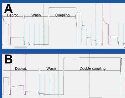
Figure 2: UV traces at 301 nm from synthesis of JR-10 using PyOxim. (A) Standard cycle with double deprotection and single coupling. (B) Difficult deprotection and coupling, automated adaption to three deprotection steps and automated repetition of coupling.
