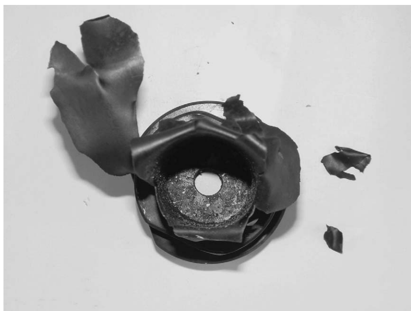
Fig. 8. 6-Cl-HOBt, Koenen test at 8.0 mm.
