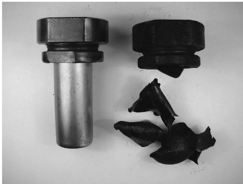
Fig. 5. HOBt with 50% water, Koenen test at 2.0 mm.
