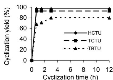
Fig. 1 Comparison of three coupling reagents (HCTU, TCTU, and TBTU) at different cyclization times in the synthesis of cyclo(SVFRGD).
